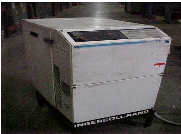
INGERSOLL RAND SSR-EP10, 10 HP AIR COMPRESSOR, 230V-3PH
