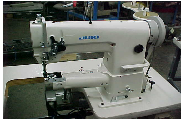
JUKI LS-321N, CYLINDER ARM NEEDLE FEED
