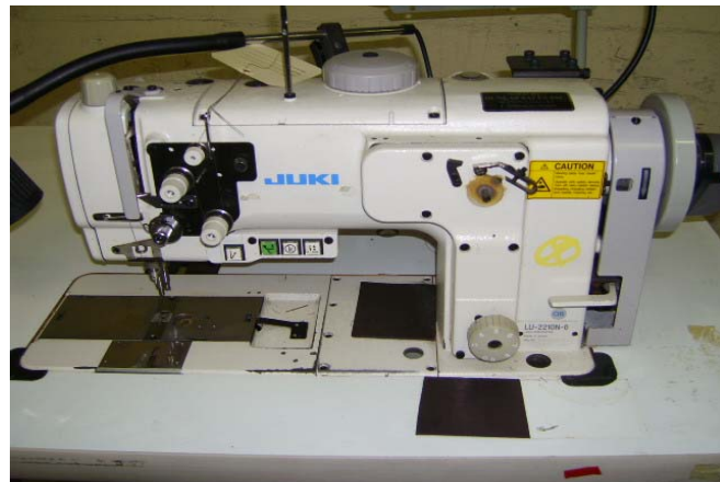
JUKI LU-2210-6, SINGLE NEEDLE LOCKSTITCH, WALKING FOOT, W/POSITION, TRIM, AUTO BACKTACK, & AUTO FOOTLIFT. (ERGO STAND)
