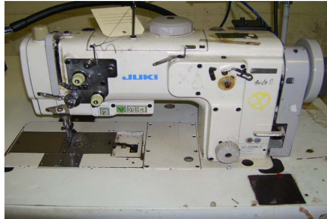
JUKI LU-2210-7, SINGLE NEEDLE LOCKSTITCH, WALKING FOOT, W/POSITION, TRIM, AUTO BACKTACK, & AUTO FOOTLIFT. (ERGO STAND)
