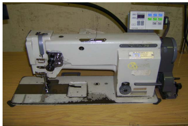
MITSUBISHI LU2-4410, SINGLE NEEDLE LOCKSTITCH, WALKING FOOT, W/POSITION, TRIM, AUTO BACKTACK, & AUTO FOOTLIFT. (ERGO STAND)
