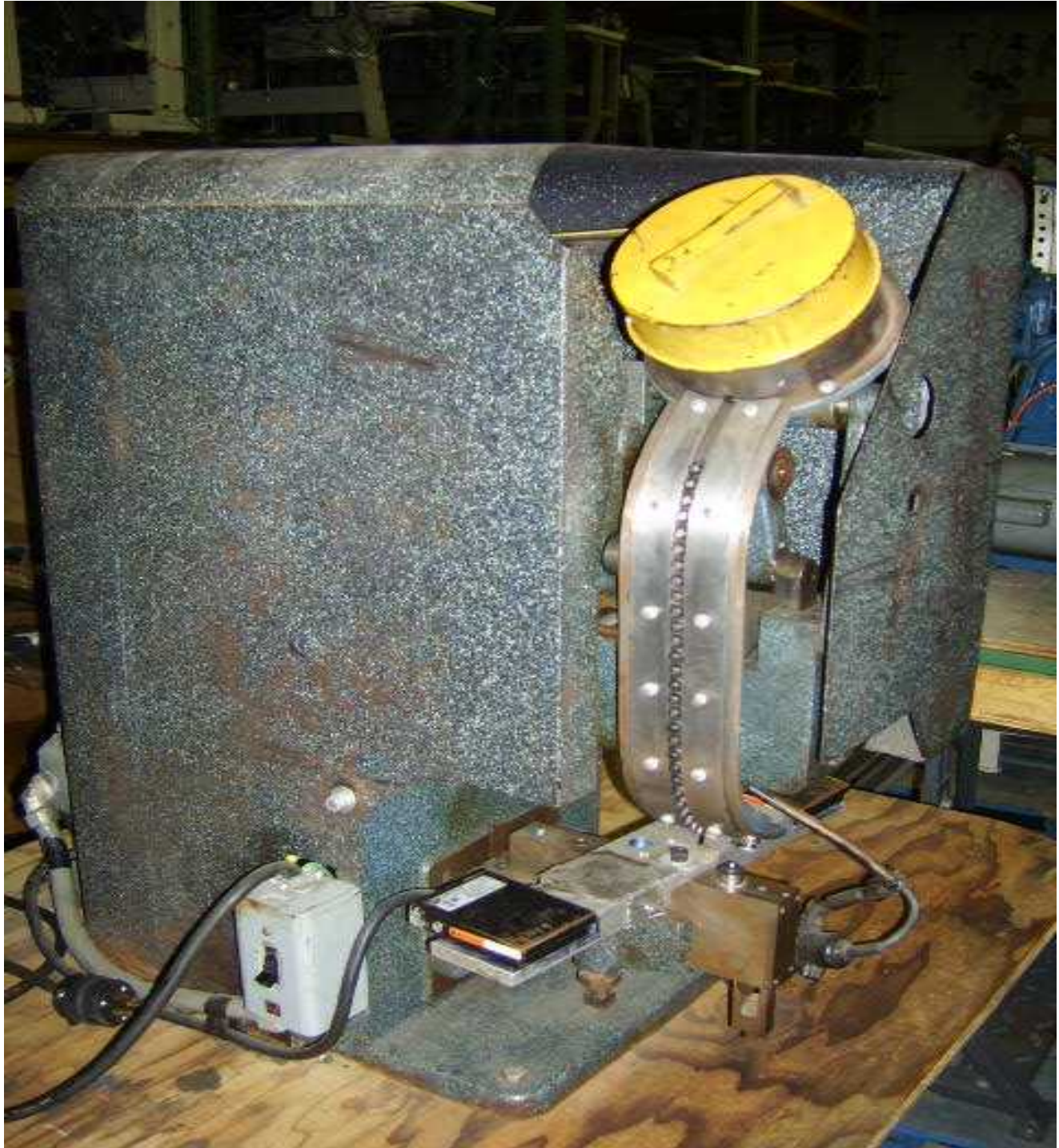
USM MODEL # WT, SINGLE HOPPER, HAND FEED WASHER. (SET-UP ON # 2 GROMMET)
